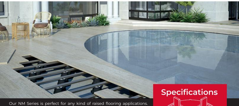
Our NM Series is perfect for any kind of raised flooring applications. When installed on a slopping surface, shims or the slope compensator can be placed on the pedestal head to ensure a level support surface. The slope compensator can add up to 1% of slope. NM pedestal can adjust from 1" – 39" without the need for pedestal bracing.
